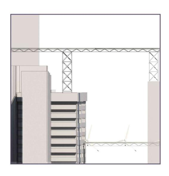
ENSURING 10 - 15 METER PRIVATE DISTANCE FROM EXISTING FACADE. HORIZONTAL BEAMS USED TO SUPPORT LONG SPAN STRUCTURES.
